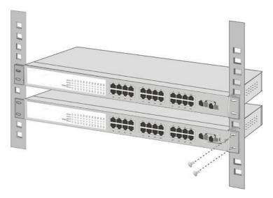
Figure 2-4 Mounting the Switch in a Rack
